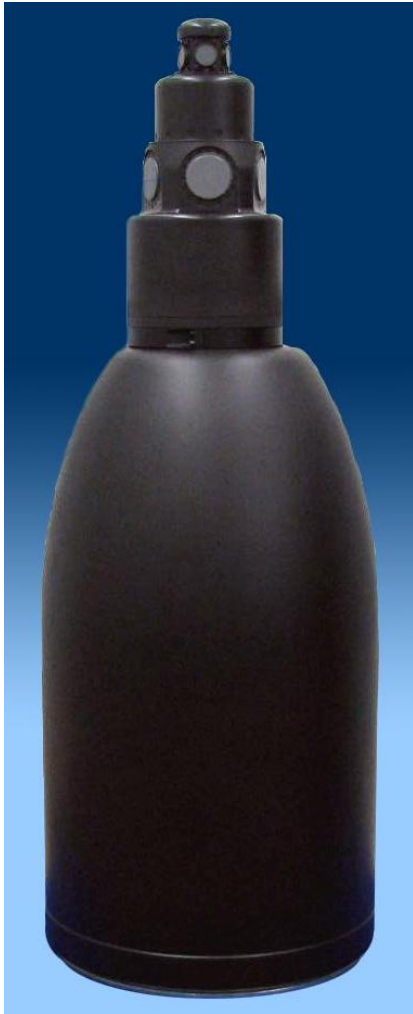
Figure 2.1 Photograph of fully integrated SIGINT Assembly with ELINT sub-system on top and COMINT sub-system below.
